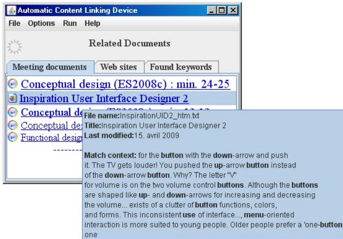
Fig. 3. Snapshot of AMIDA ACLD’s widget UI, showing the tab with the list of relevant documents at a given moment, with explicit document and snippet labels. Hovering over a label displays the metadata associated with the document, as well as excerpts where the keywords were found. Tabs displaying detected keywords and retrieved websites are also available.
