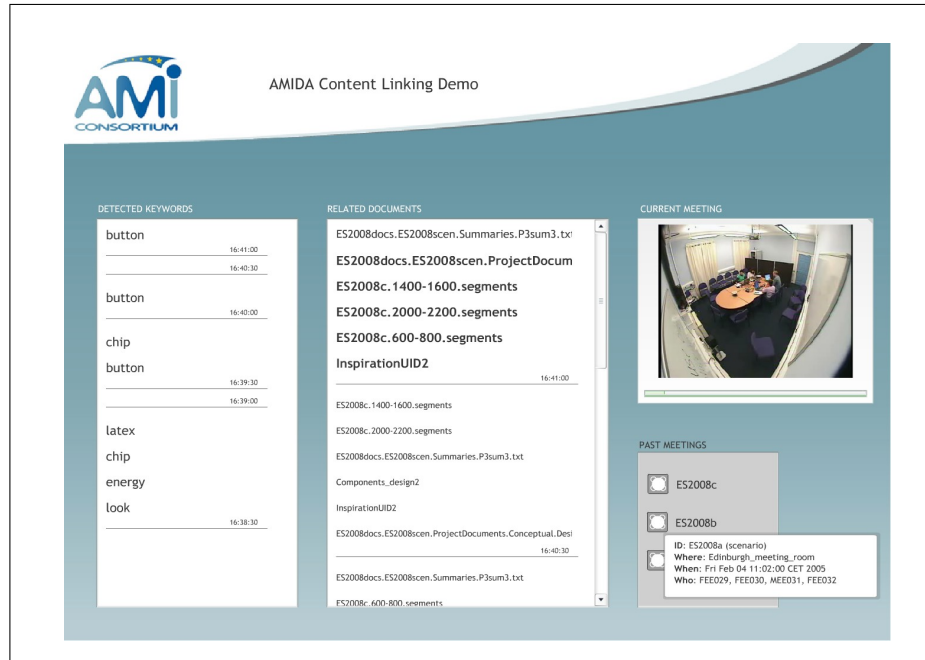
Fig. 2. Snapshot of AMIDA ACLD’s user interface over meeting ES2008d. Left column shows recognized keywords with timing, central column shows relevant documents (with font size coding for importance), and bottom-right box shows a list of the previous meetings of the series, giving access to their contents.
